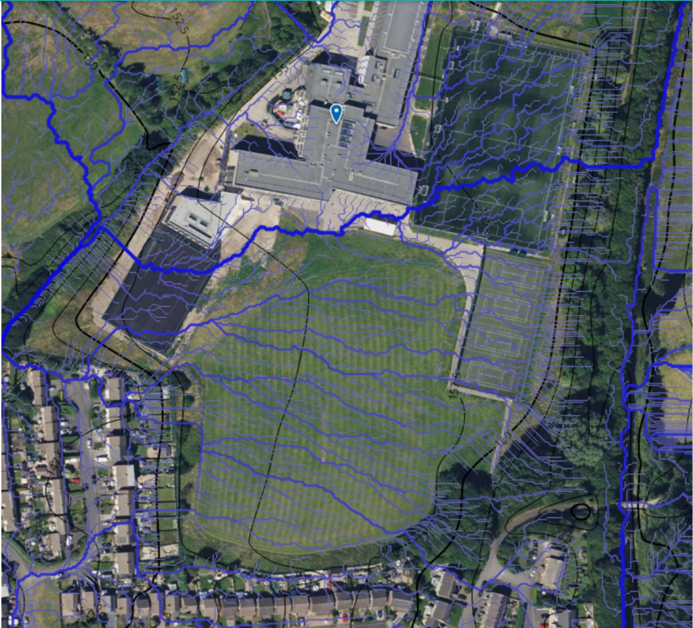
Figure 5 – Surface water mapping using Scalgo shows surface water flow across the site flowing from the east to the west down with the natural fall of the land. The surface water flood risk on the MUGA comes from flow from higher ground and woodland to the NE of site.
