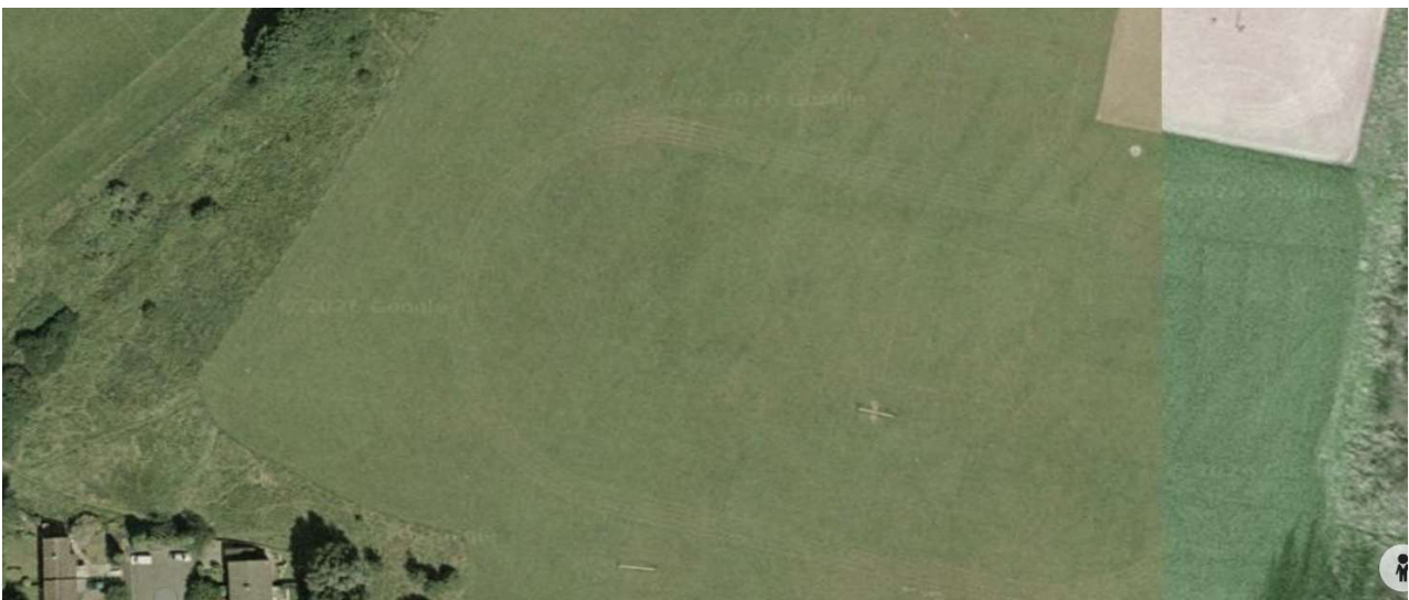
Figure 9 – Google Earth image dated 2003 showing same pipe drainage lines at approx. 6m spacings. However, further development of the site to include a larger 3G on the east side and a new MUGA of the west side would likely have disrupted the existing pipe network.
