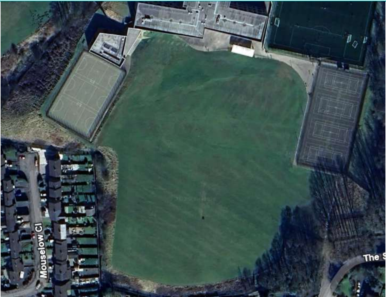
Figure 8 – Google Earth image dated March 2025 of southern field showing pipe drainage lines at approx. 6m spacings. These same lines are apparent in a Google Earth image dated 2003 – see below.
