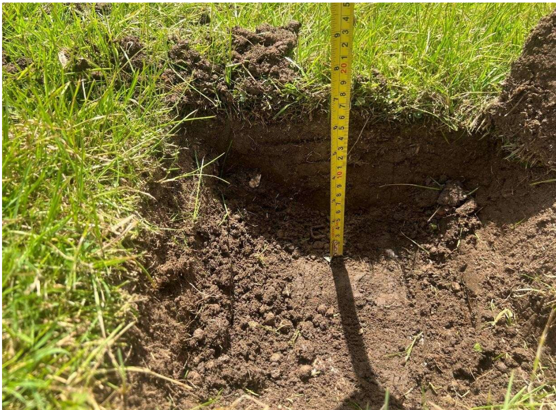
Photo 4: Excavated trial pit
